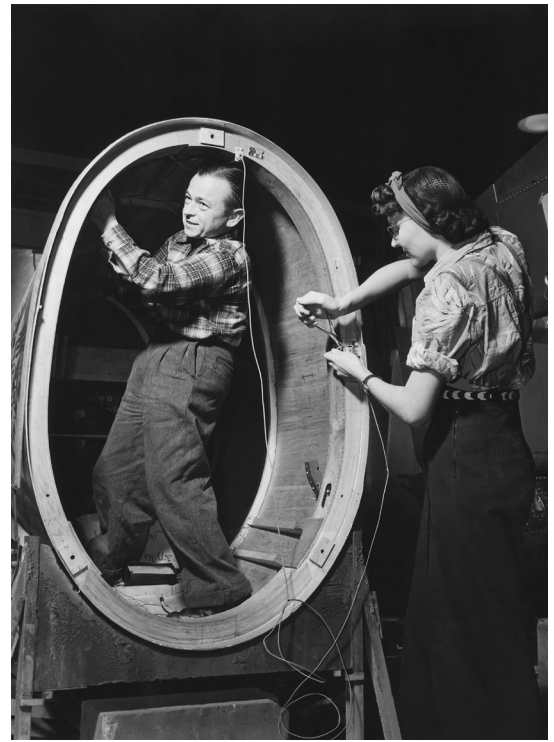
A small man installs control wires inside the fuselage of a 'Valiant' basic trainer while a woman works standing outside. Vultee Aircraft Downey Plant, Ca. 1942–43. (Shutterstock)
